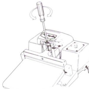
Sealing pressure can be easily adjusted with a screwdriver.
